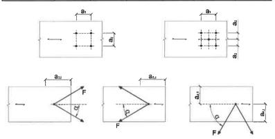
A.2.1 Definition of spacing, end and edge distances in the plane surface of the cross laminated timber.
