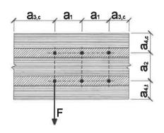
Definition of spacing, end and edge distances in the edge surface of the cross laminated timber. For A.2.2 screws in the edge surface, a1 and a3 are parallel to the CLT plane face, a2 and a4 perpendicular to CLT plane face.
